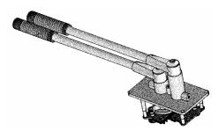
This dual stacked lever controller provides full follow up control of the dual steering gear systems commonly found on Push Boats. These vessels are a regular sight on the Mississippi and adjoining river systems. One steering gear controls the steering rudders aft of the propellers and the other the flanking rudders forward of the propellers.
